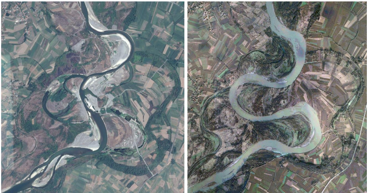
□ Figure 54 and 55: Example of the lower Bosna. Left: situation 2015, right: situation in 2003. Intensive sediment extraction has caused degradation of the river channel. [21].
