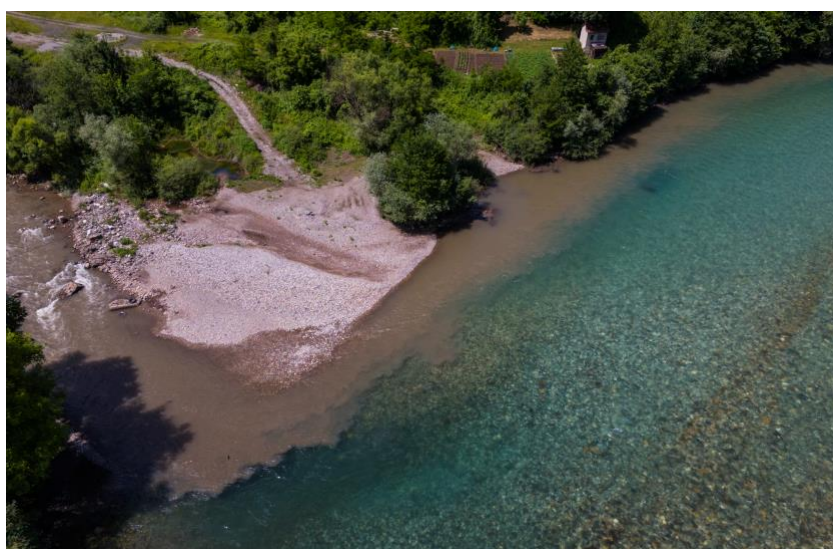
Fig. 6. Heavy input of fine sediment into the Bistrica River during the spring spawning season of the Danube salmon – caused by hydropower construction – disrupts successful reproduction of the resident fish community. © Bruno D'Amicis
