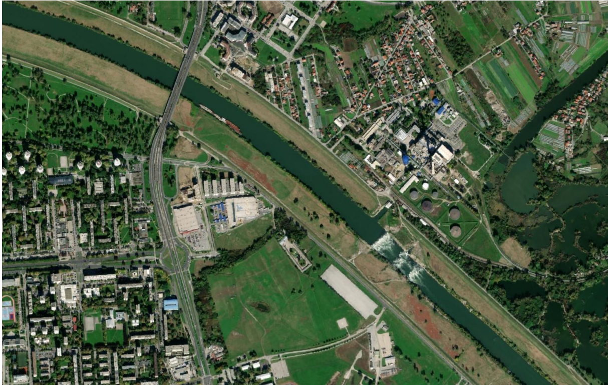
Figure 6: The Sava in Zagreb, strongly altered, with trapezoid cross section, detached floodplains and ramp for retaining cooling water, Class 4 (extensively modified) (Source: Bing Virtual Earth).
