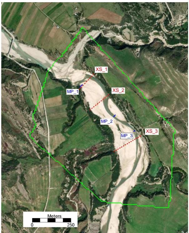
Figure 1. Aerial view of Shushica site 1; MP = measurement Profile (blue line); XS=cross-section (dashed red line); green polygon = DTM boundary
