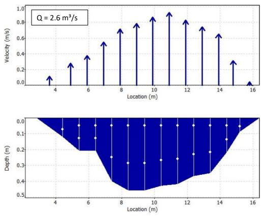
Figure 10. Measured mean flow velocity (top) and measurement profile MP\_1 (bottom) at Shushica 2.
