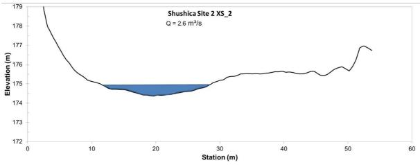
Figure 12. Cross-section XS\_2 including measured water level at a discharge of 2.6 m<sup>3</sup>/s
