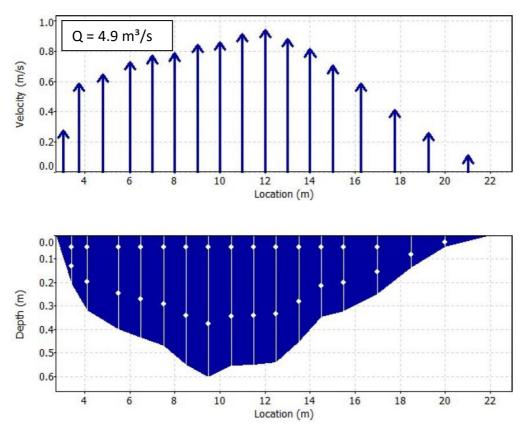
Figure 3. Measured mean flow velocity (top) and measurement profile MP\_2 (bottom) at Shushica 1.
