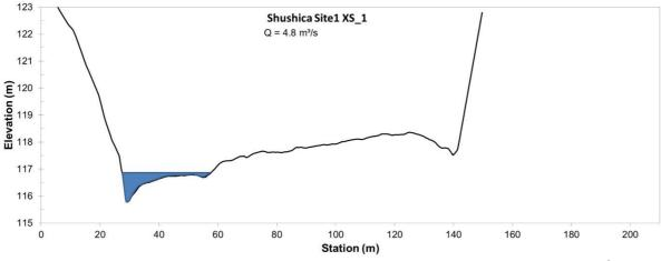
Figure 5. Cross-section XS\_1 including measured water level at a discharge of 4.8 m<sup>3</sup>/s
