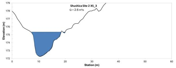
Figure 13. Cross-section XS\_3 including measured water level at a discharge of 2.6  $m^3/s$
