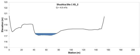
Figure 6. Cross-section XS\_2 including measured water level at a discharge of 4.8 m<sup>3</sup>/s
