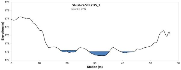
Figure 11. Cross-section XS\_1 including measured water level at a discharge of 2.6 m<sup>3</sup>/s
