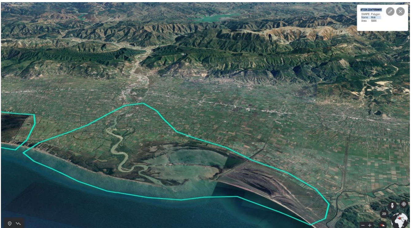
Often, deltas are affected by many hydropower plants in the catchment (reservoir in the background) and intensive sediment dredging along the lower courses (where the river enters the plain). But this image also shows the coast's vulnerability and the vital function of deltas for coastal protection. (Google Earth 2023).
