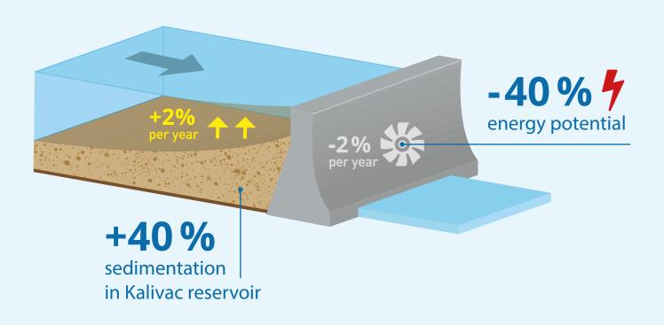
More sediments, less energy: The Kalivaç reservoir would constantly fill up with sediments, leading to a 2% loss of energy potential each year. After 20 years, the power plant would lack 40% of its original capacity.
