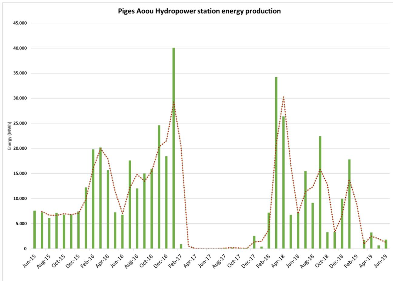
Figure 26. Electrical energy production from the Piges Aouu Hydropower station, between June 2015 and June 2019.<sup>21</sup>
