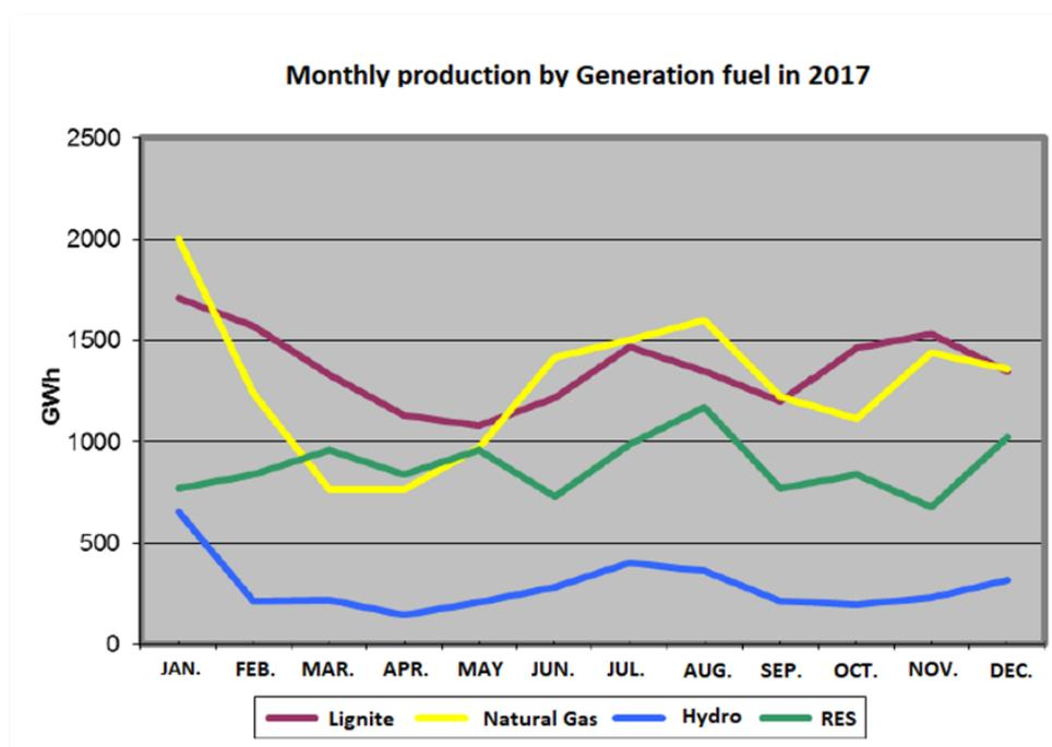
Figure 2. Monthly electricity production by generation fuel in Greece in 2017 (RAE, 2018)
