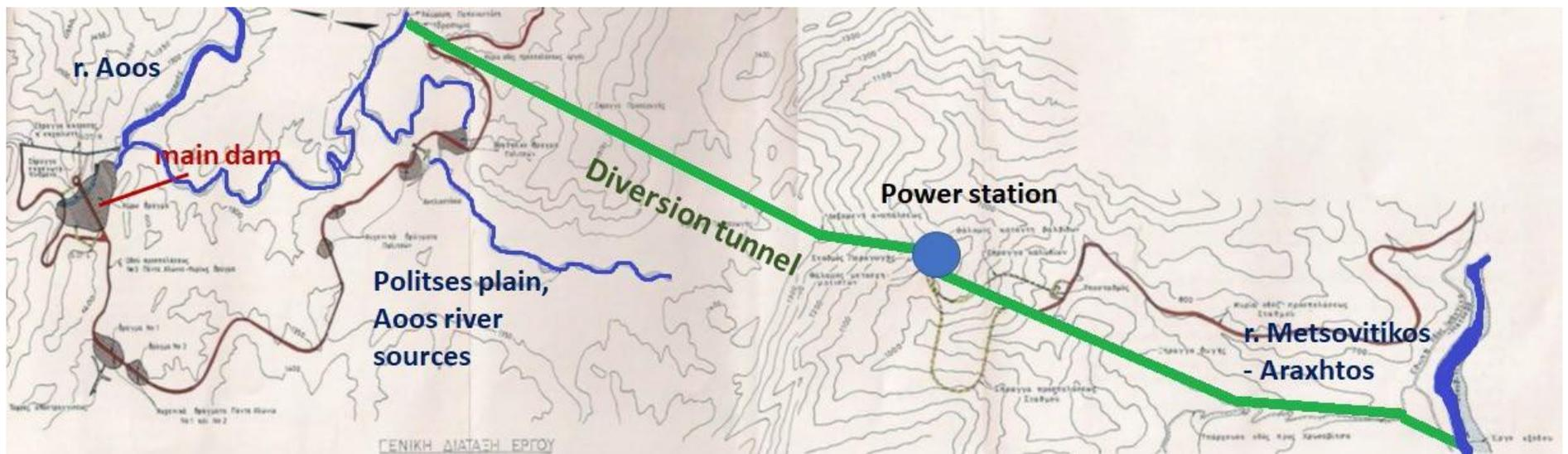
Figure 29: General diagram of the Piges Aooou hydro-system.
