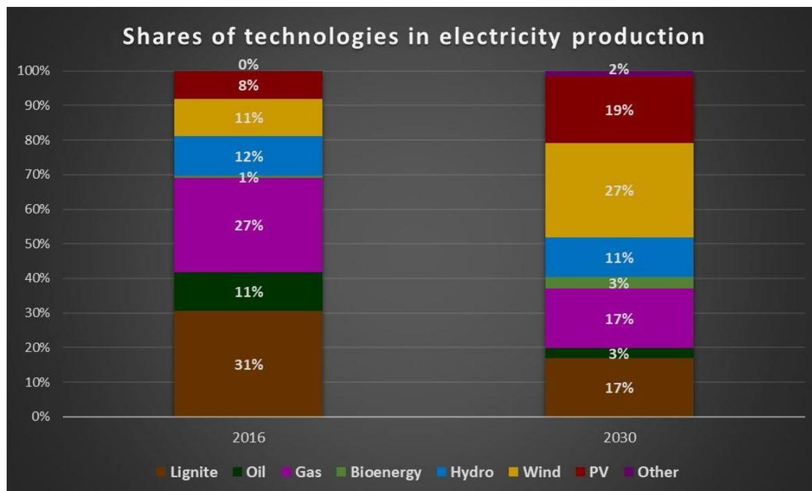
Figure 18. Shares of various technologies in electricity production in Greece for the year 2016 and the corresponding estimation for 2030 (YPEN, 2018).
