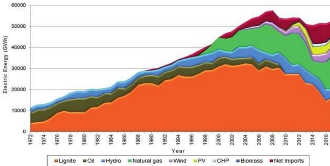
Figure 3. Evolution of electricity generation by fuel in the Interconnected System of Greece since 1972, including the net result of imports-exports (Roumpos et al., 2018).
