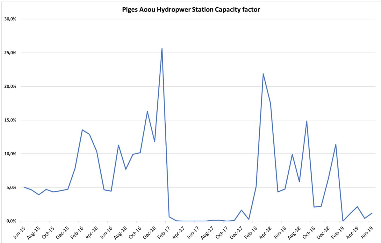
Figure 27. Capacity factor of the Piges Aouu Hydropower Station, between June 2015 and June 2019.
