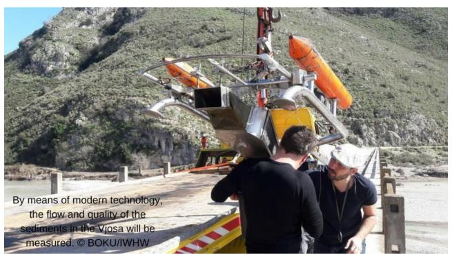
**Assessment of sediment transport in the Vjosa has started!** The University of Natural Resources and Life Sciences Vienna (BOKU), together with the Polytechnic University of Tirana, have started an assessment of sediment transport in the Vjosa river in Albania. They are measuring the amount of gravel, sand and fine sediments the river transports into the Mediterranean Sea each year. The results will allow conclusions about the efficiency of the projected hydropower projects. MORE
