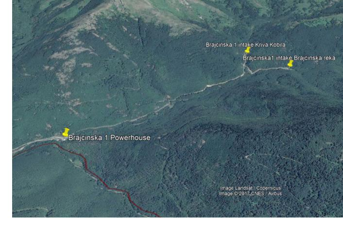
on the main, Brajcinska river. The pipes, following the access road, are approximately 2500 m long including the section that goes to the Kriva Kobila intake.
