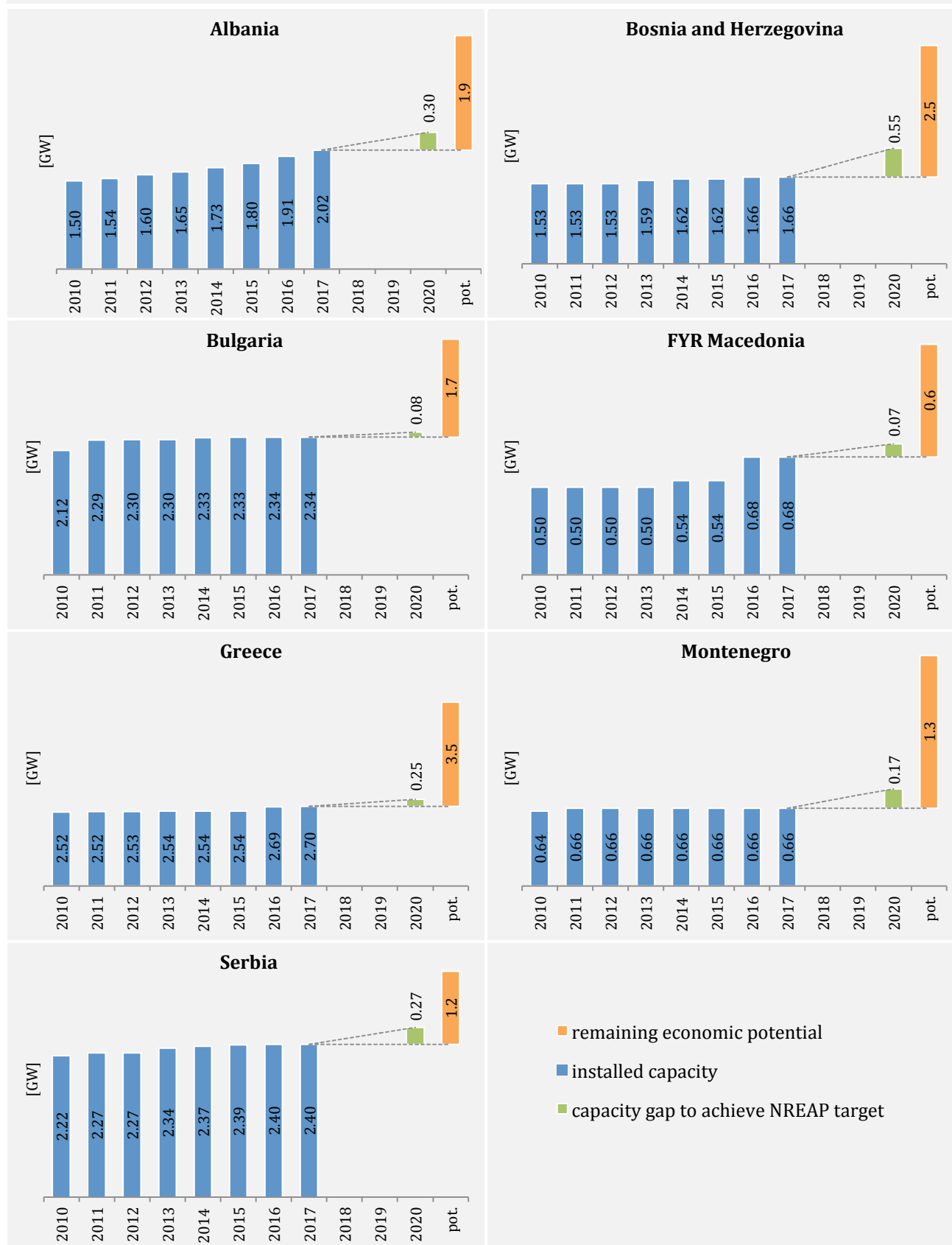
Fig. 13: Hydropower capacity development 2010 - 2017, NREAP 2020 target and economic potential
